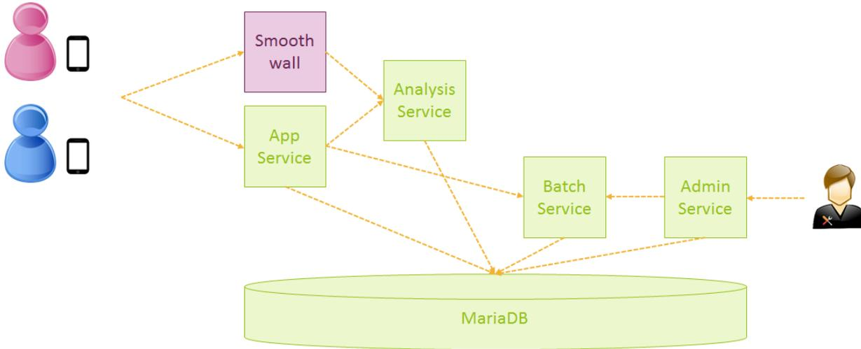
All Yona services use the same database schema and they share a cache, synchronized through Hazelcast. Communication between the services (e.g. from the app service to the analysis service or the batch service) is always through HTTP.
